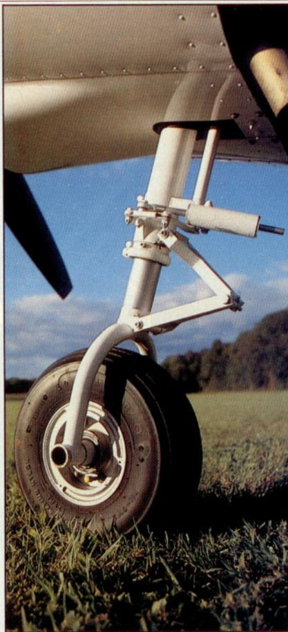
*When extended in flight, the nose gear strut disengages from the rudder, making the pedal controls very light.*
